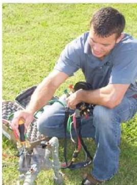
A backflow preventer is usually tested with a device called a *differential gauge*. This gauge uses hoses attached to the various test ports of the reduced pressure zone and checks to be certain that the check valve springs as well as the relief valve spring are not fouled and are working properly.
