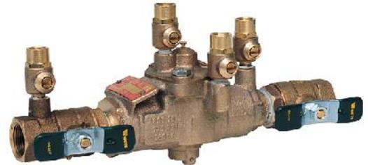
Any visible water discharge from this type of backflow preventer device is usually an indication that either of the two check valves is *'passing'* (leaking past their shutoff seats) or the relief valve itself is faulty.
